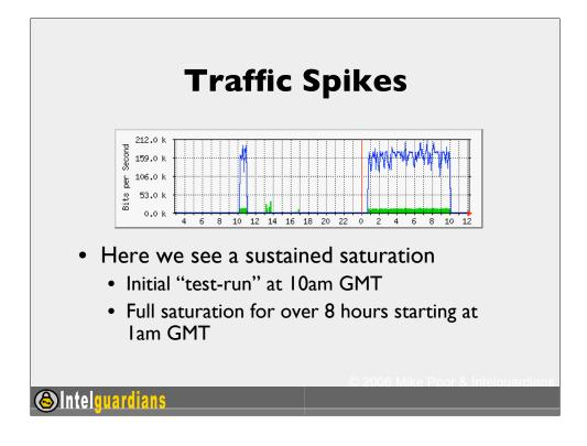
Here we see a traffic spike (actually two) using MRTG, the Multi-router traffic grapher. This tool collects SNMP data from network devices and displays hourly, daily, monthly and yearly graphs.
