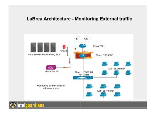
In this diagram see an architecture deployment model for Labrea. LaBrea sits on the DMZ network and traps worms as they enter the network. This is great for worm research, as well as practicing being a good net citizen. On the next slide we see a different deployment strategy, as to allow Labrea to watch for outbound scanning coming from internal hosts.
